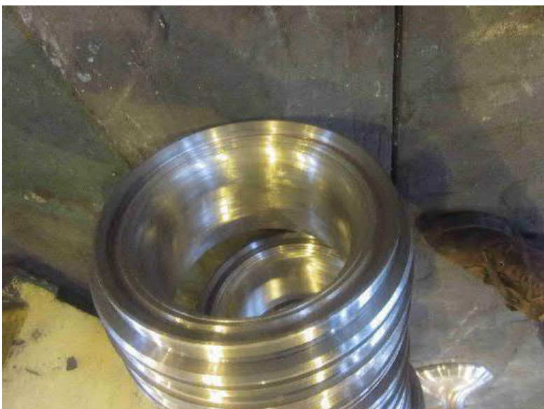
Valve seat contact surface view after recondition
