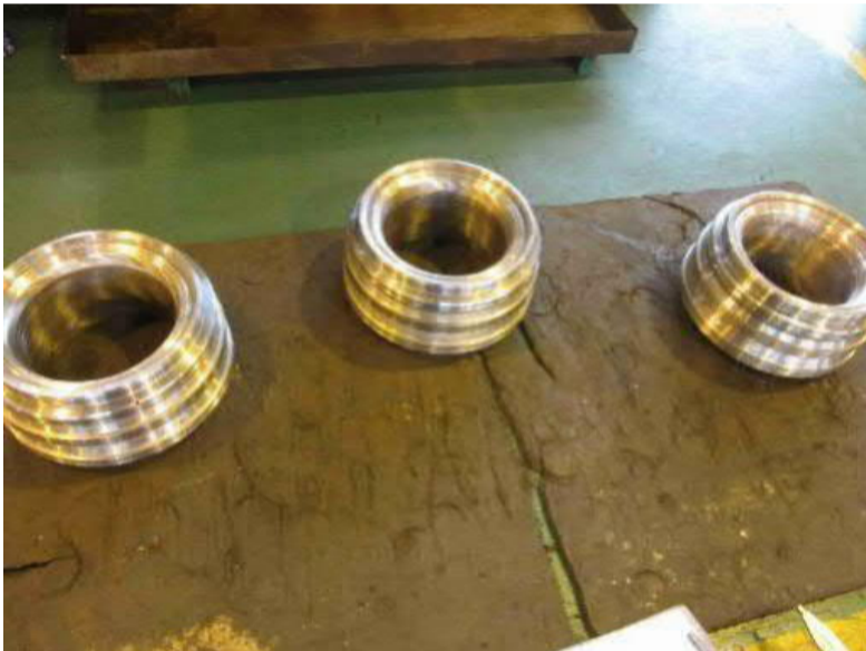
Over view of valve seats after recondition
