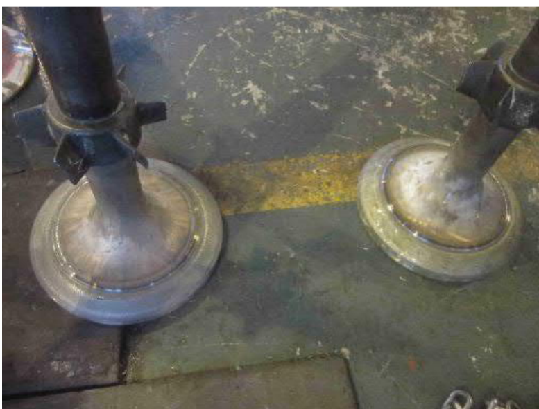
Contact surface be cladded with Stellite material
