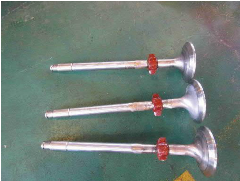
Valve spindle over view after recondition
