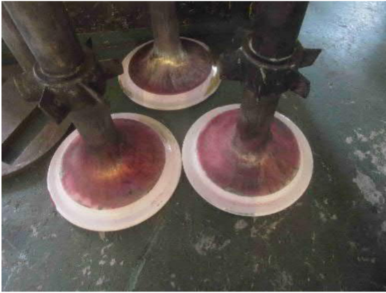
Rough machined of valve spindles
