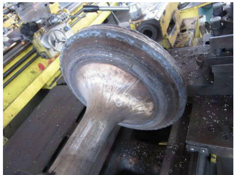
Valve spindle machined zone be re-built up
