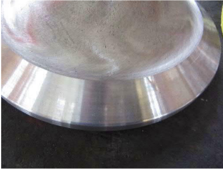
Valve spindle contact surface close view
