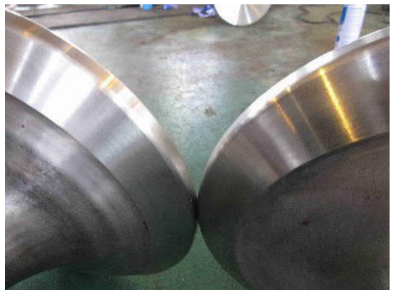
Valve spindle contact surface close view
