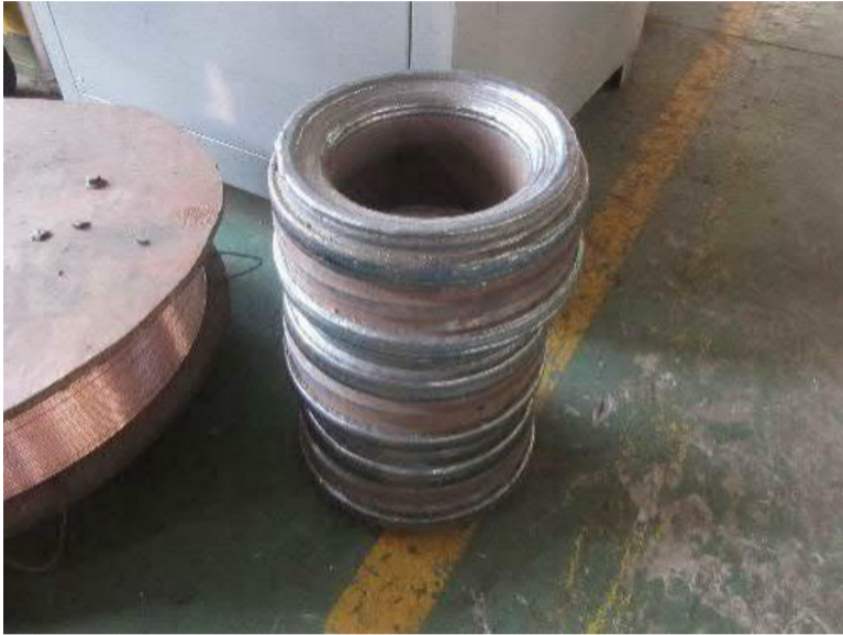
Valve seat machined zone be re-built up
