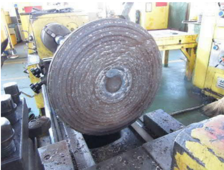
Valve spindle machined zone be re-built up
