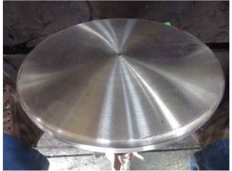
Valve spindle bottom disc view after recondition
