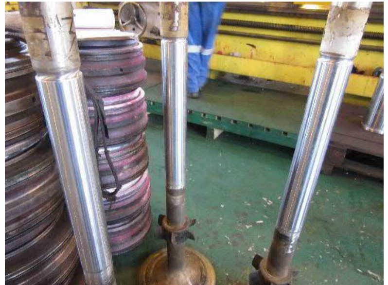
All 4PCs valve spindle guide stem were chromed
