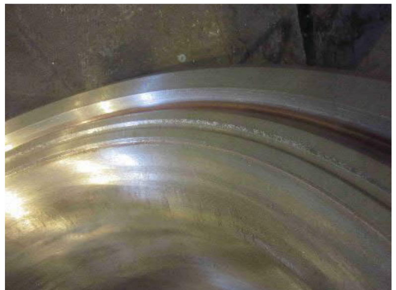
Valve seat contact surface close view
