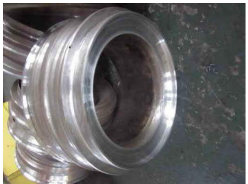
Rough machined of valve seats
