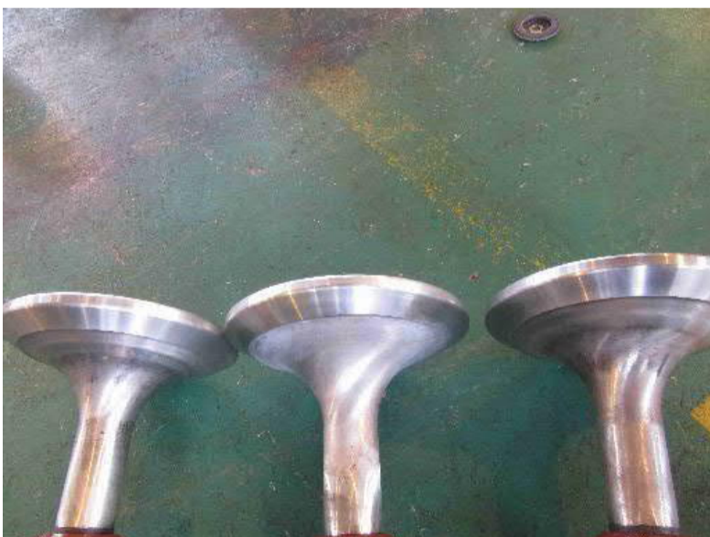
Valve spindle contact surface view after recondition
