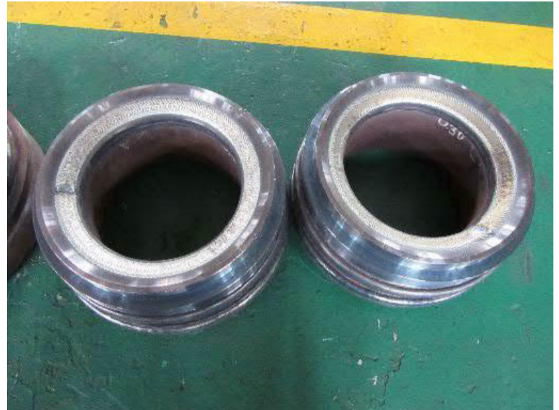
Contact surface be cladded with Stellite material
